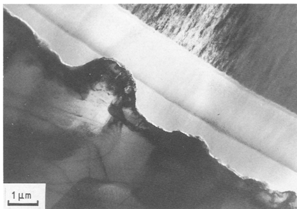
Figure 5 As-fabricated SCS-6/Ti-6Al-4V showing uneven penetration of the protective coating. (Fibre at top right.)
