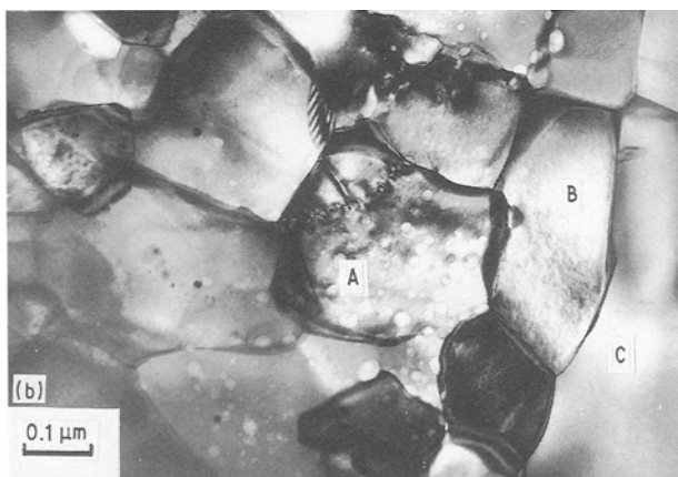
Figure 6 (a) SCS-6/Ti-6Al-4V after 3 h at 1050^\circ C showing columnar SiC grains of fibre at lower left; the remainder of reaction layer consists of individual grains of Ti_5Si_3 , Ti_5Si_4 , and TiC. (b) Extreme right-hand edge of RZ shown in (a) bounded on the right by a grain of Ti_5Si_4 (marked C). (c) EDS spectrum of crystal marked "A": analysis indicates TiC. (d) EDS spectrum of crystal marked "B": analysis indicates Ti_5Si_4 . (e) EDS spectrum of crystal marked "C": analysis indicates Ti_5Si_3 .
