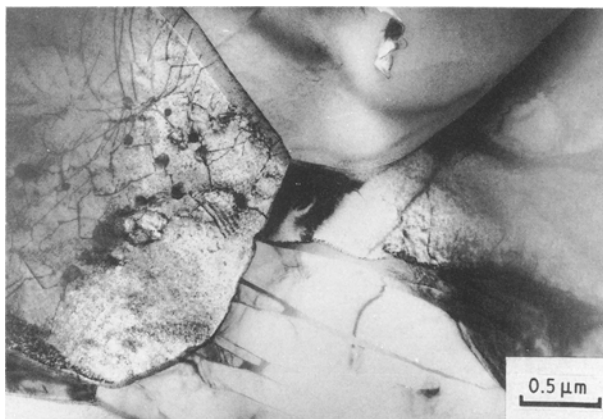
Figure 8 TiC crystals (at left and right) in matrix of SCS-6/Ti-6Al-4V, showing mottled appearance and internal dislocations and precipitation.
