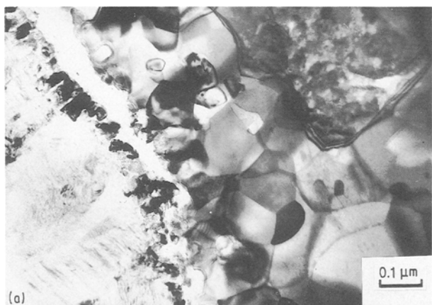
Figure 6 (a) SCS-6/Ti-6Al-4V after 3 h at 1050^\circ C showing columnar SiC grains of fibre at lower left; the remainder of reaction layer consists of individual grains of Ti_5Si_3 , Ti_5Si_4 , and TiC. (b) Extreme right-hand edge of RZ shown in (a) bounded on the right by a grain of Ti_5Si_4 (marked C). (c) EDS spectrum of crystal marked "A": analysis indicates TiC. (d) EDS spectrum of crystal marked "B": analysis indicates Ti_5Si_4 . (e) EDS spectrum of crystal marked "C": analysis indicates Ti_5Si_3 .
